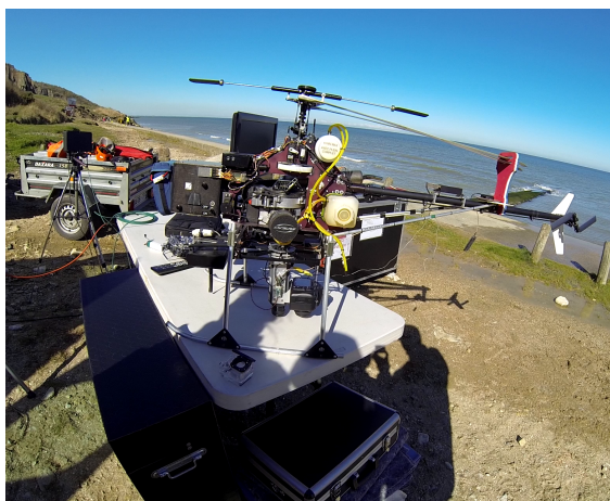
Figure 2. Copter 1B UAV used for the acquisition (Photo : R. Antoine/TeleDeTAC project).
