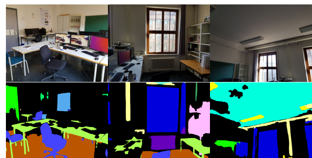
Figure 2. Figure 2: Exemplary results of using our trained DeepLabv3+ model for inferencing the images of an interior room.
