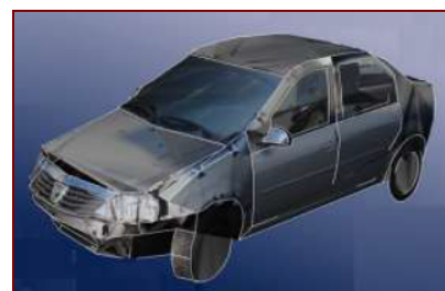
Figure 1. 3D Model created in PhotoModeler Scanner software with textures (Oniga et al., 2016)
