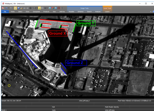
Figure 10. Stratosphere Tower, imagery chipped from WorldView-1 and marked with chosen ground origin (yellow marker) and coordinate axes. A second chip is also used, collected from a perspective such that the layover of the tower is to the right.
