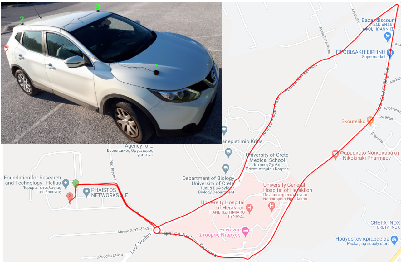
Figure 1. Closed route traversed in a counterclockwise direction overlaid on a Google street map. Start and end points are indicated with green and red pins, respectively. The inset image shows the antennas of the three u-blox receivers attached on the car used.
