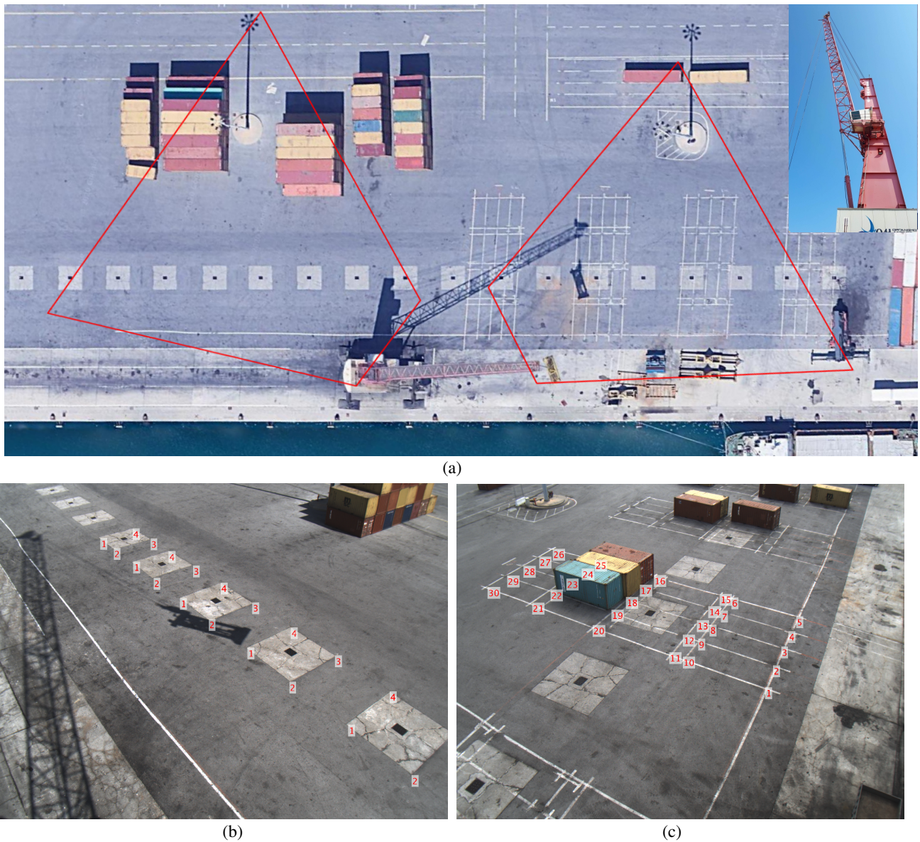
Figure 3. (a) Non-orthorectified satellite view of the port quay with the crane in the bottom middle and the inset image. The two red quadrangles correspond to the intersections of the quay's plane with the camera frustums of the images in (b) and (c) [the position of the crane shown in image (a) does not coincide with that from which images (b), (c) were taken]. (b), (c) Views of the quay from the camera installed on the crane. The image in (c) was obtained from the reference location and has the employed GCPs superimposed. The four extremal junctions used for the world to image homography estimation are GCPs 1, 5, 26 and 30. Image (b) is a view from the camera after the crane has rotated about 120^\circ in a counterclockwise direction. The GCPs shown are used for pose verification.
