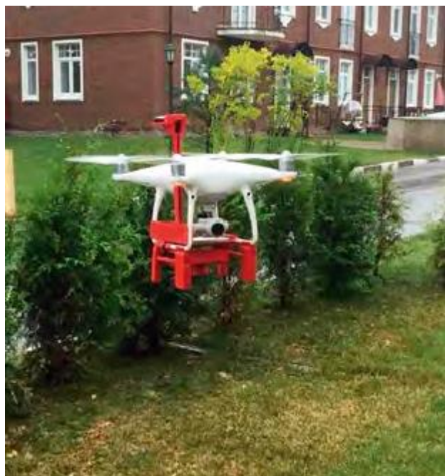
Figure 15. Special suspension for RedEdge multispectral sensor.
