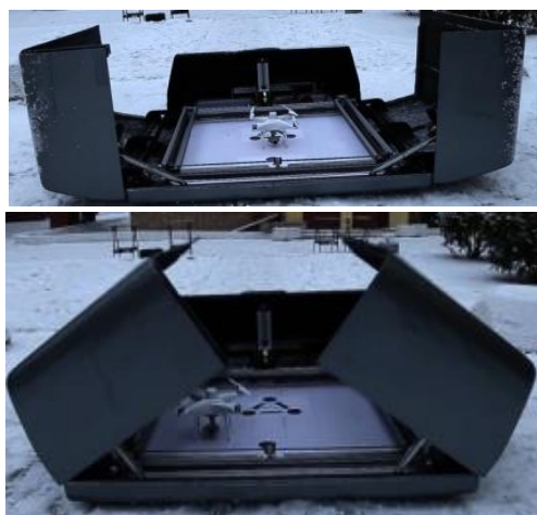
Figure 3. Stationary complex - Installed on a car trailer, trunk. The UAV lands in the box.
