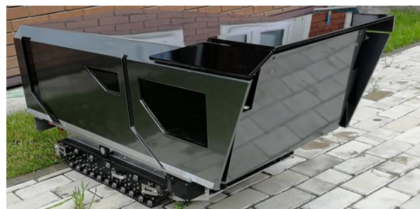
Figure 4. Mobile complex on tracked course - radius of autonomy 1000 m. speed 5 km/h. UAV lands on the ground
