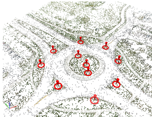
Figure 6. Eleven GCPs established in the study area to ensure that the road's mesh model was generated with a correct scale
