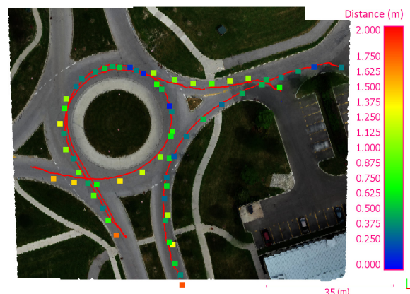
Figure 13. Distance of the estimated position of the test vehicle in the low-altitude video from its measured position using RTK GNSS; the trajectory includes two tours around the roundabout.
