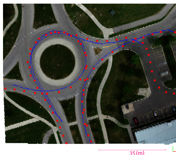
Figure 12. Estimated position of the test vehicle using the proposed vision-based approach in the low-altitude video (blue) and its measured position using real-time kinematic GNSS (red)
