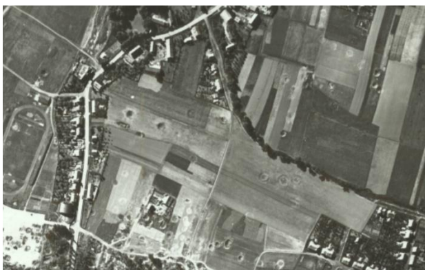
Figure 14 Identification of unexploded ammunition in an image of 1945
