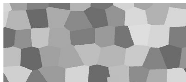
Figure 12 Mask used for inlaying images into the final orthophotomap
