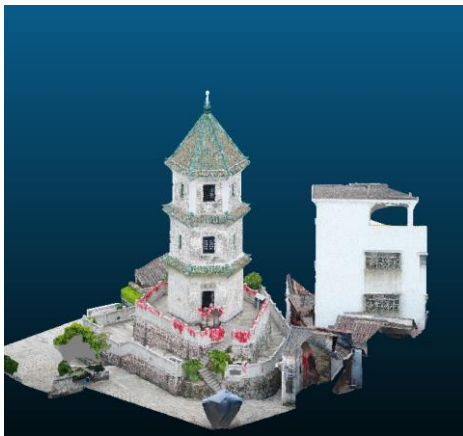
Figure 2. Point clouds reconstructed from UAV photogrammetry for the Wenfeng pagoda located in Guangdong Province, China
