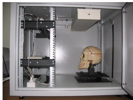
Figure 2. Digital photogrammetric system for automated textured skull 3D models generation
