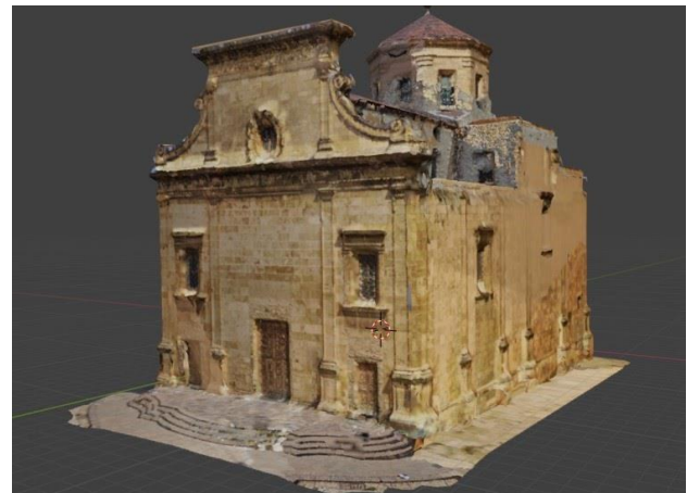
Figure 7. The textured mesh model of the church obtained following the first solution after editing operations in Blender.
