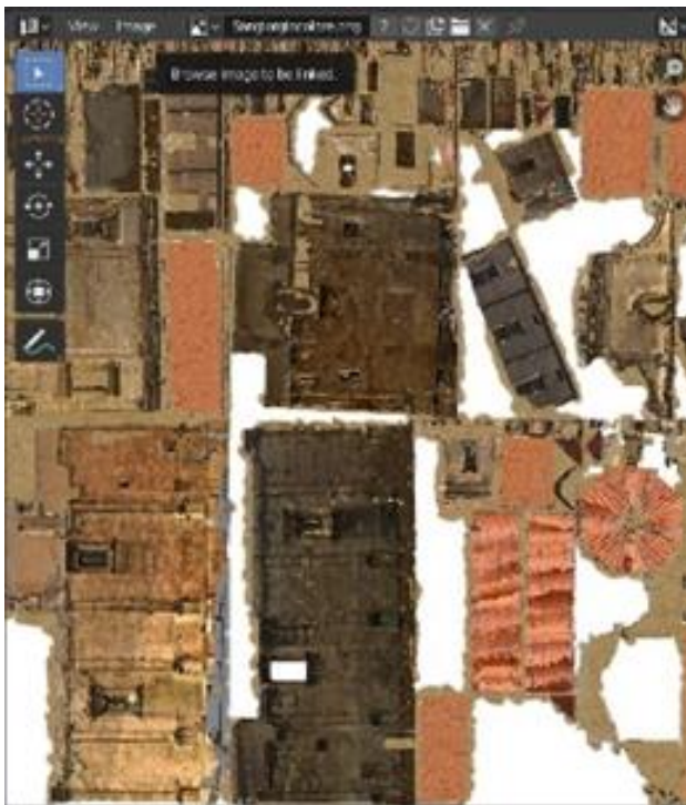
Figure 9. UV mapping operation on the texturization of the 3D model in the second solution.
