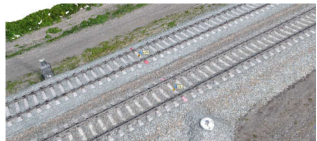
Figure 4. A fragment of a dense point cloud with control points placed by pairs
