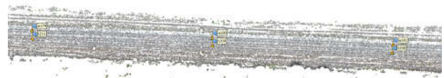
Figure 3. A fragment of the photogrammetric model with control points placed by pairs every 200 m
