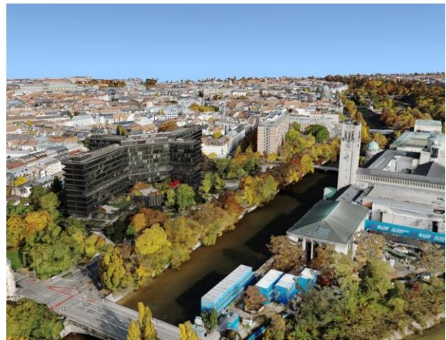
Figure 12: Automatic result of 3D Mesh, produced by Melown Technologies, using CityMapper-2 data with 5 cm GSD
