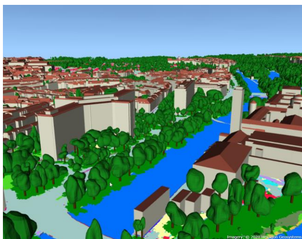
Figure 11: Automatic result of 3D land use and LOD2, produced by Melown Technologies, using CityMapper-2 data with 5 cm GSD
