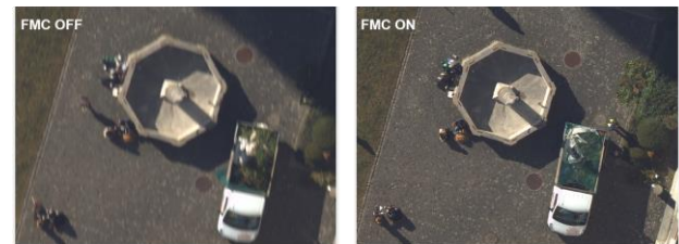
Figure 2: Leica MFC150 with FMC off/on - showing the benefit of FMC for long exposure at low sun angle (1/200 sec at 120 km)
