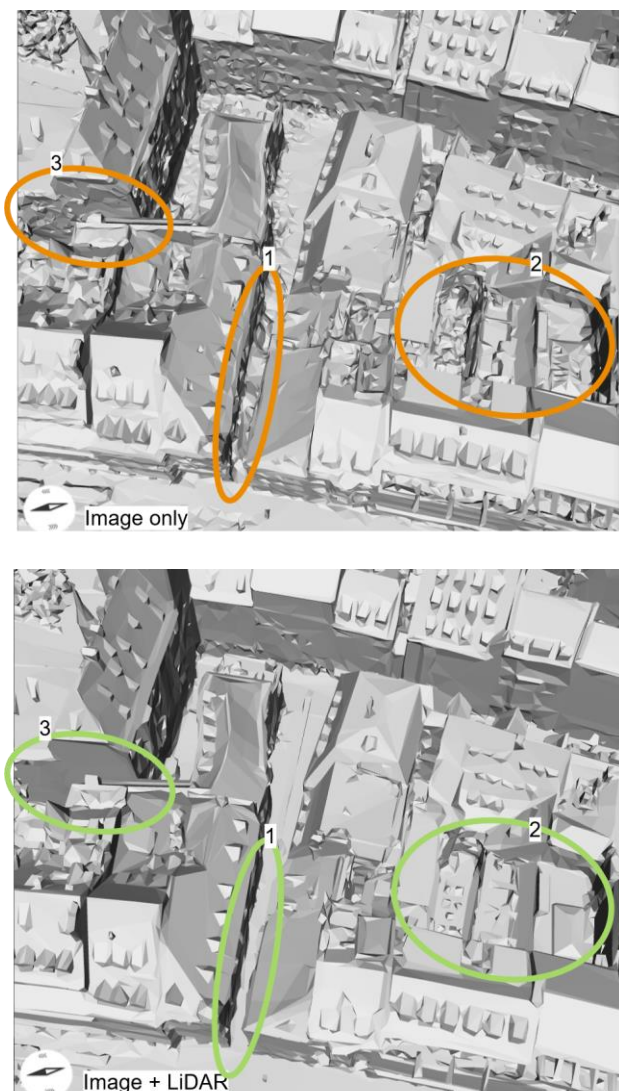
Figure 14: Comparison of 3D Mesh from image only (top) and image + LiDAR (bottom) approach. 3D mesh generated by Melown technologies from CityMapper-2 data, 5 cm GSD
