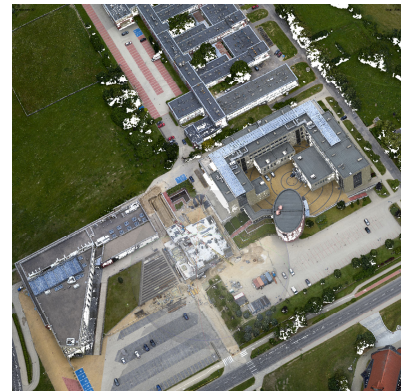
Figure 5. Visualization of a part of the point cloud generated in the Agisoft Metashape application.
