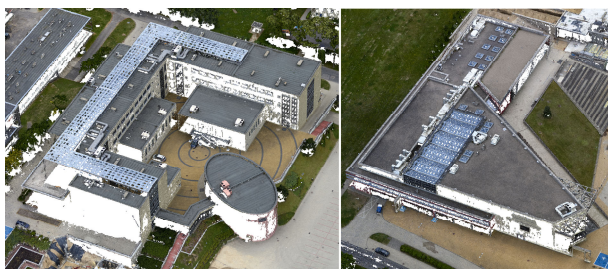
Figure 4. Image-based point clouds generated in Agisoft Metashape software.
