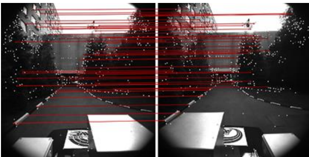
Figure 2. The result of the algorithm for matching interest points.
