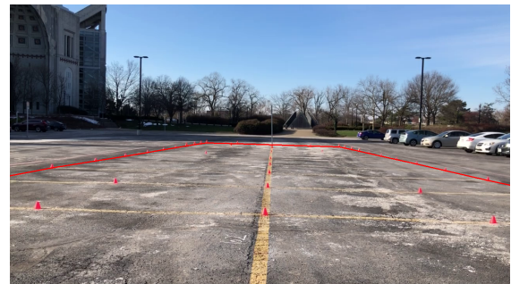
Figure 7. Camera view from monocular camera mounted on the vehicle. Red polyline is the margin of ROI. HE-Net will be activated only objects whose bottom points are within ROI. Cones on the ground are markers for homography estimation.
