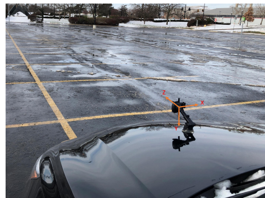
Figure 5. Dataset collection platform with predefined camera coordinates with respect to vehicle moving forward direction, x , y and z axis point at right, down and forward directions.
