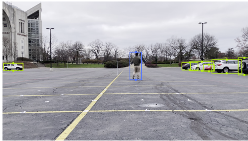
Figure 3. Object detection output generated by the detection network in the form of a bounding box: b_{i,j,1}, b_{i,j,2}, b_{i,j,3}, b_{i,j,4} . Marked two points (middle bottom and middle above) of the bounding box represent object bottom and top, such that the object height is the length of the line connecting these two points.
