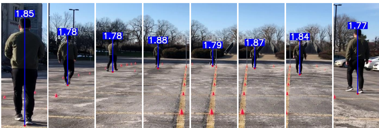
Figure 9. Person's estimated height over frame. Texts above the person are heights in meters.
