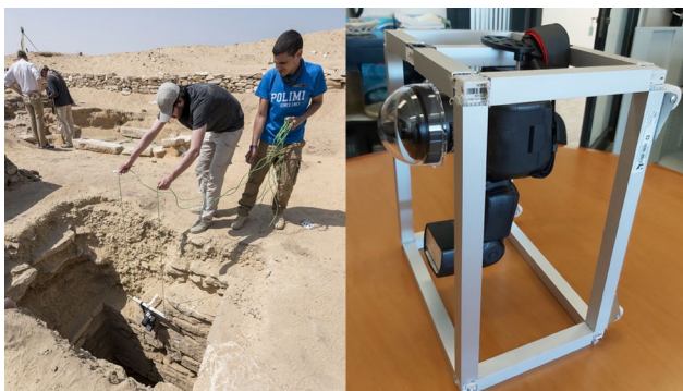
Figure 10. On the left the survey of a shaft in Saqqara in 2018, on the right the design of a wired wheeled cage to survey vertical shafts, designed and assembled in 2020.
