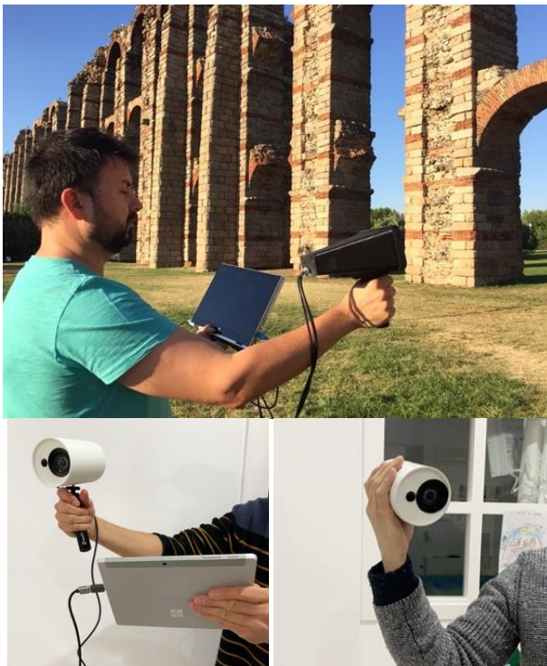
Figure 1. Evolution of the design of the prototypes. First prototype while scanning the Roman aqueduct of "Los Milagros" (above). Last version of the prototype optimising the design and ergonomics by carrying it on a handle (bottom left) and carrying it directly by hand (bottom right).
