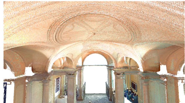
Figure 3. Point cloud of Palazzo Mazzonis atrium. Scan: M. C. López González; processing: F. Natta.
