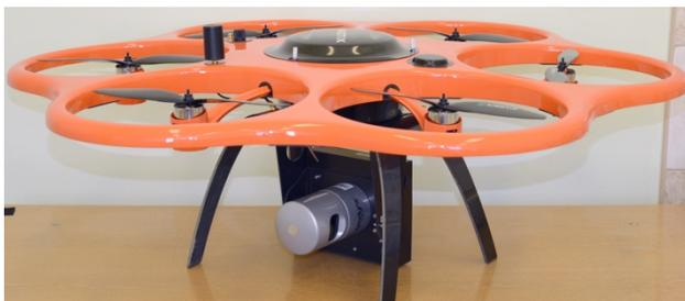
Figure 3. Aibot X6 V2 with Velodyne HDL-32E laser scanner.
