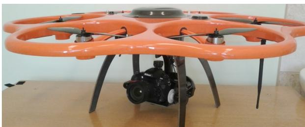
**Figure 2.** Aibot X6 V2 with Nikon D800 camera.
