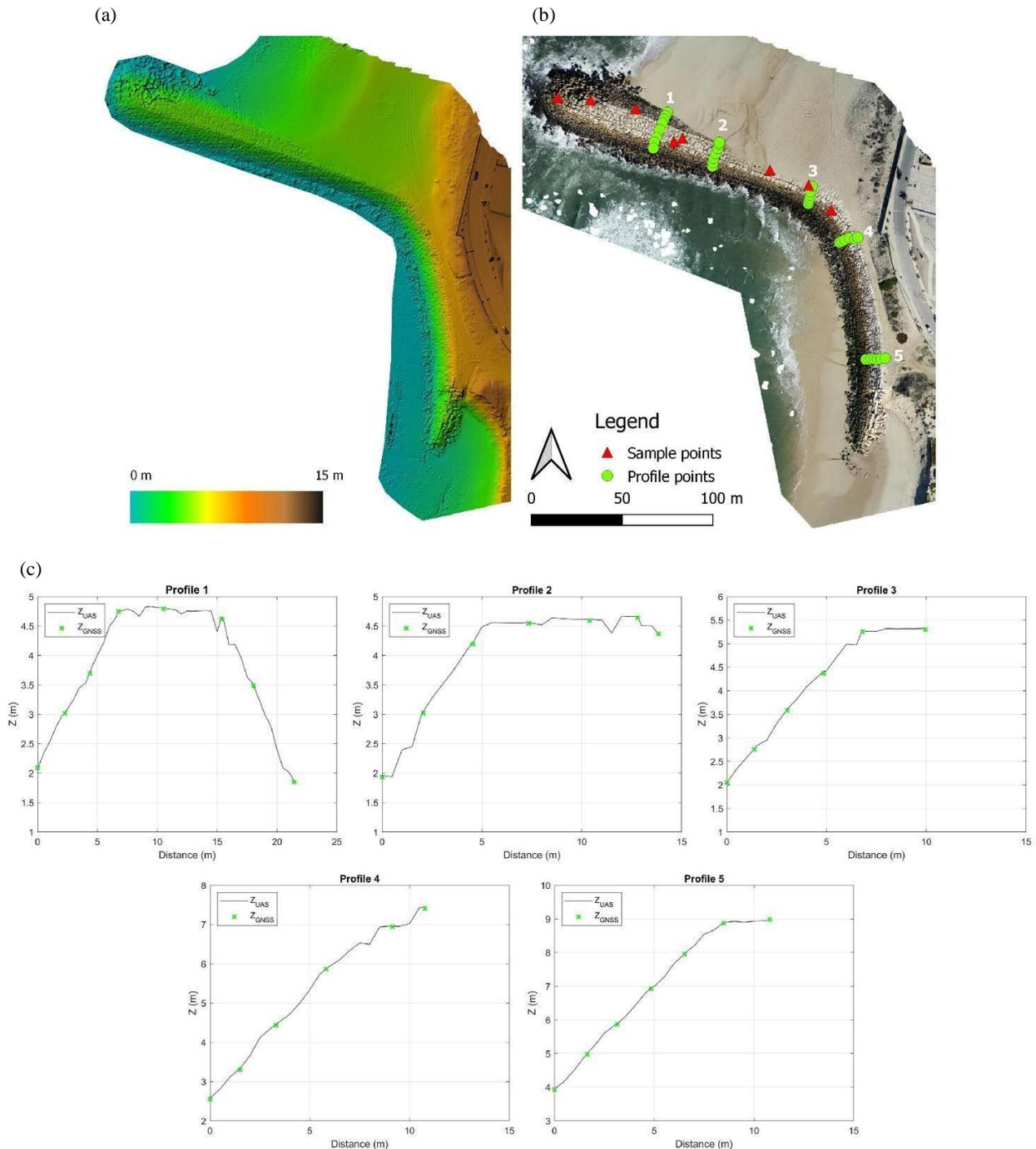
**Figure 2.** Products obtained DJI Phantom 4RTK and generated in Agisoft Metashape. (a) Digital Surface Model (DSM); (b) Orthophoto and the point used in vertical accuracy analysis. (c) The profiles were obtained with GNSS (green crosses) and UAS DSM (black lines with 50 cm bin spacing).
