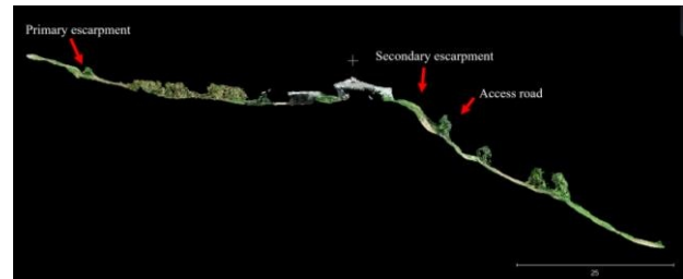
Figure 7. Profile 1 exported to AutoCAD® Civil 3D – Side view.
