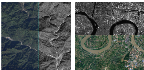
Figure 1. Example of multimodal images with direct georeferencing. (a) Google (Left) and GaoFen-2 Panchromatic (Right) images. (b) Google (Nether) and Sentinel-1 SAR (Upper) images.
