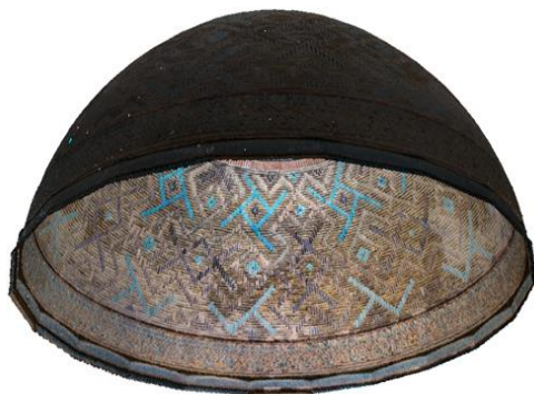
Figure 1. The ideal point cloud of İnce Minareli Madrasa's dome created by raw images.
