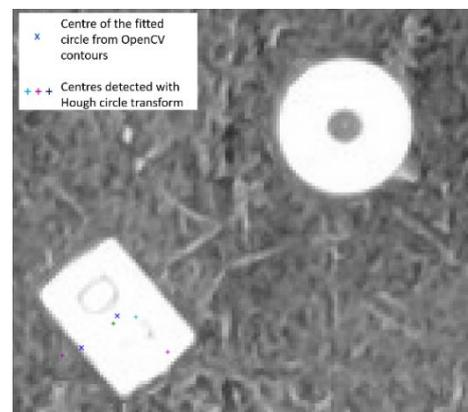
**Figure 7.** Example of false positives mis-detected with the OpenCV algorithm due to a relatively oblique viewing angle.
