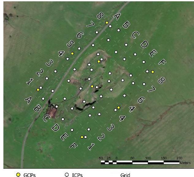
**Figure 1.** Test field target distribution at Wards Hill quarry, Northumberland, UK, Map data: Google Earth 2021.
