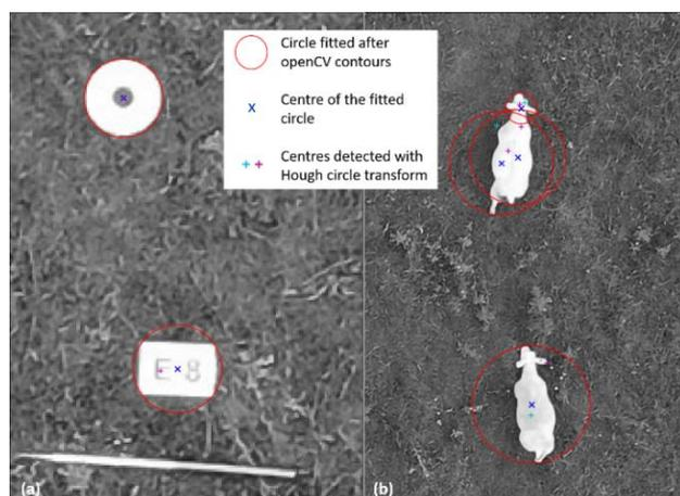
**Figure 6.** Examples of correct and erroneous target detections, the latter removed from the final outputs via the developed automated OpenCV workflow.
