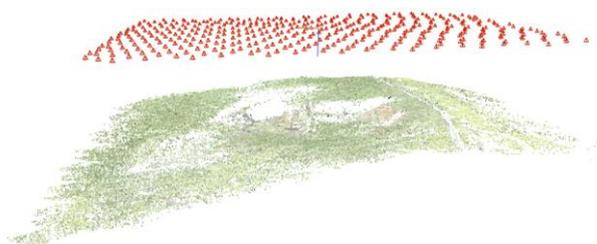
**Figure 8.** Sparse cloud calculated with COLMAP and Key.Net local features.
