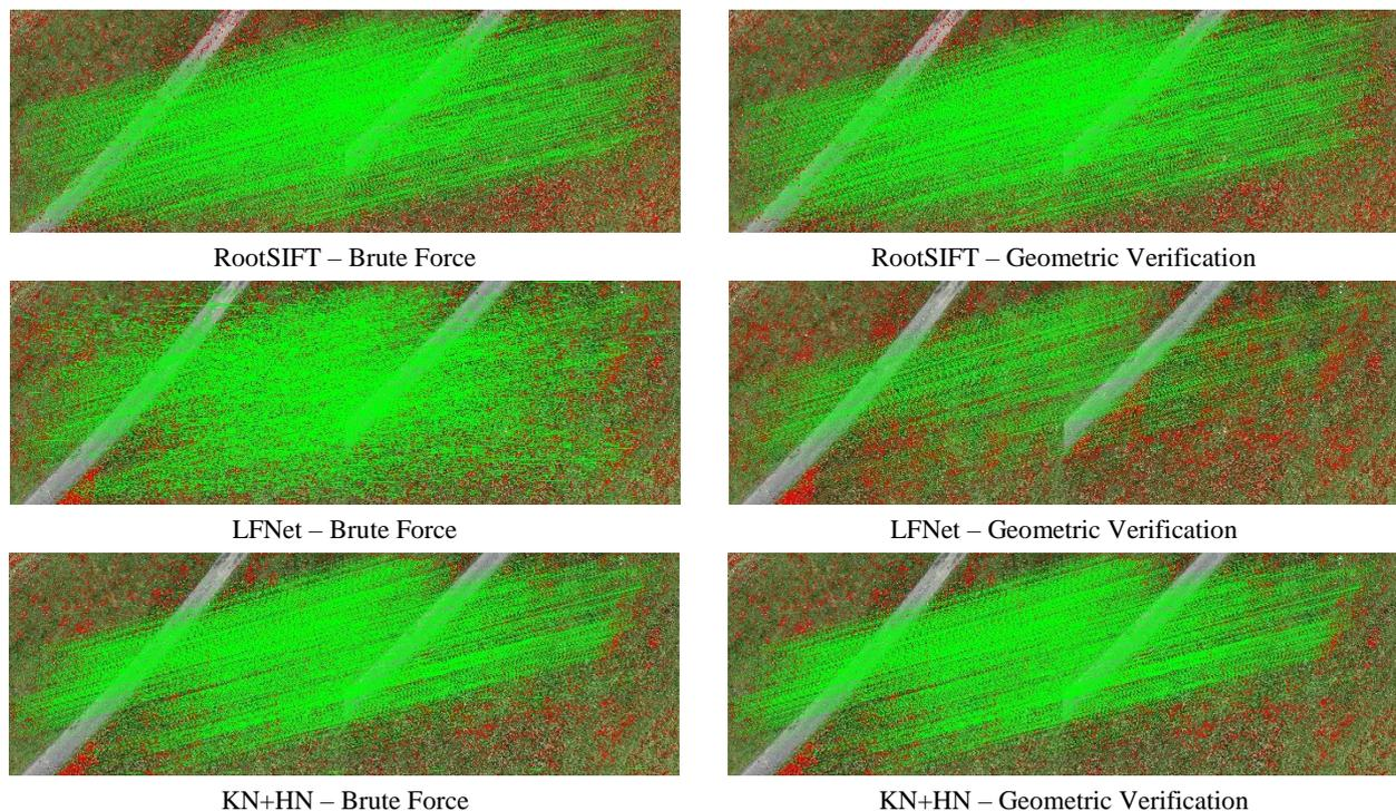
**Figure 9.** Image matching comparison before and after geometric verification.
