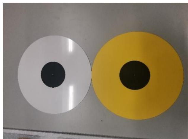
**Figure 2.** 300 mm diameter targets - CPs (l) and GCPs (r).
