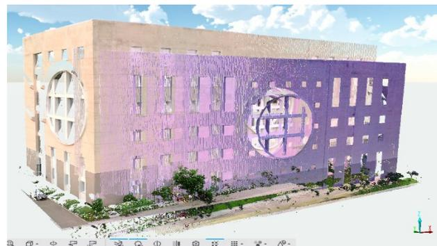
Figure 11. 3D point cloud RGIPT Academic building 2 process data by SCENE software
