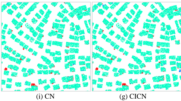
Figure 11. Examples of building detection. ■, TP; ■, FN (mis-detections); ■, FP (over-detections)
