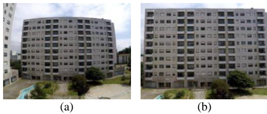
Figure 1. Example of GoPro images in standard mode (a) and linear mode (b).
