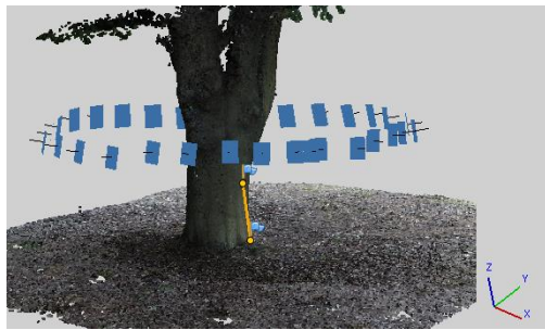
Figure 3. Reconstructed model of the tree, with the measurement of a check distance.
