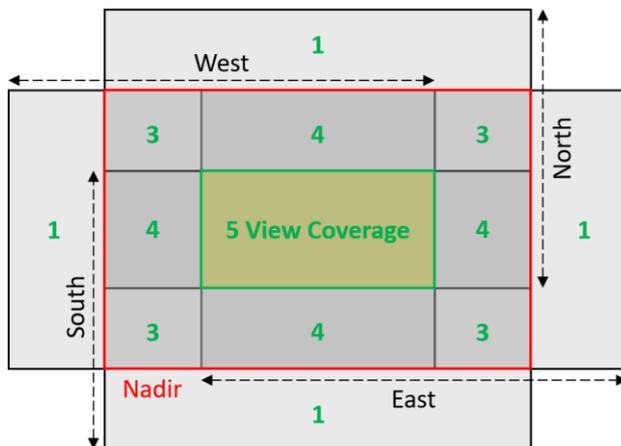
Figure 2. Illustration of an oblique sensor's block layout, with a central (usually large) five-view coverage and partial coverage near the block edges. If flown in East-West direction, left/right or backward/forward sensors images are looking North/South or East/West, respectively.
