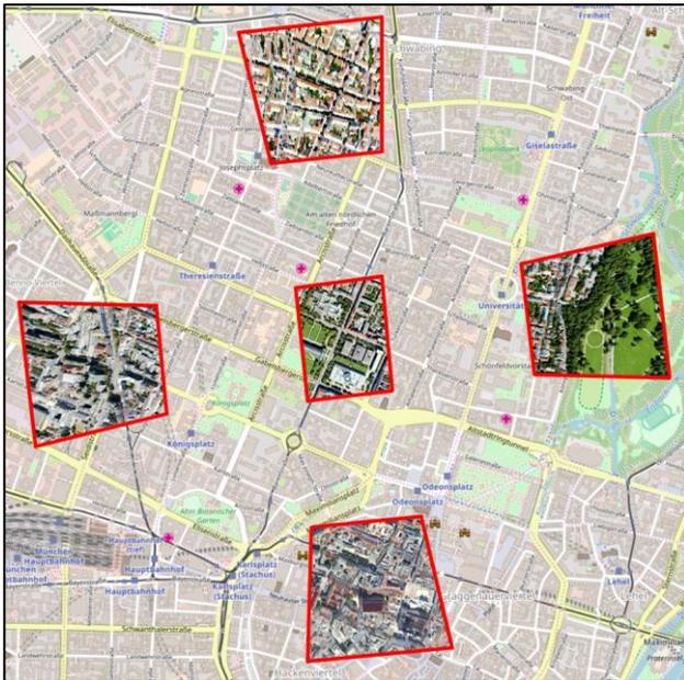
Figure 1. Example of Leica CityMapper-2S nadir and oblique ground coverage from one image take. Image data was captured over Munich, Germany, in 2021 (see also chapter 4).
