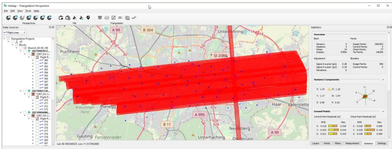
Figure 5. HxMap Workflow Manager with the AT project for the Munich Central block, showing some key statistics on the right.
