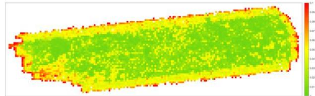
Figure 3. Color-coded visualization of the tie point standard deviation CBA layer for Munich Central, hierarchical AT. Color scale is between 0 and 0.010 m or ~ 3 GSD, with “green” areas < 1 GSD.
