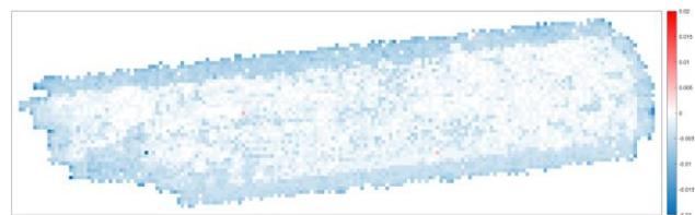
Figure 4. CBA difference between hierarchical and integrated AT for Munich Central. Color scale is -0.020 m to +0.020 m.
