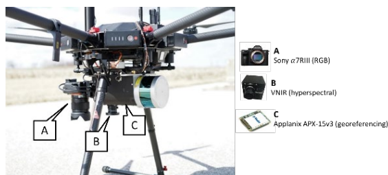
Figure 1. The UAV-based mobile mapping system and onboard sensors used in this study.
