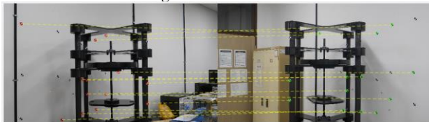
Figure 6. Matching points in frames from Camera A and Camera B after outliers were removed
