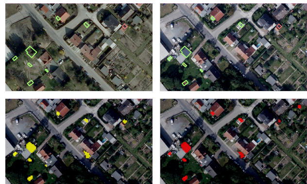
Figure 1. Change detection results using the HC + C_{building} input at \tau = 0.5 . Top row: Orthophotos from 2010 (left) and 2016 (right) with the reference classes new in green and demolished in red. Bottom row: binary change detection results for ALS-ALS (left) and ALS-DIM point clouds (right).
