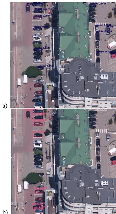
**Figure 4** Example where detection results from YOLO learned on two different image sets partially complement each other:
