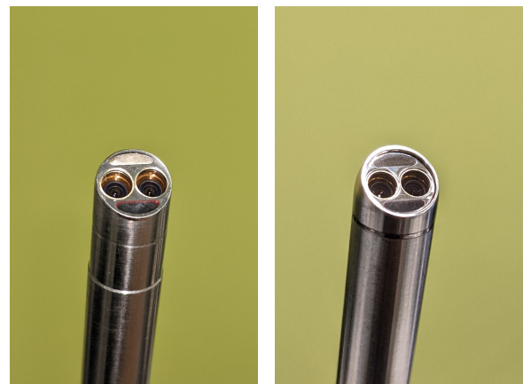
Figure 3. Tip of Einstein : on the left without the sterile cover and on the right with it.
