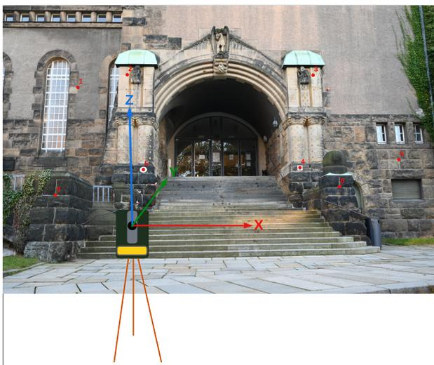
Figure 6. Coordinate system as defined for evaluating the coordinate values for the camera poses. Additionally, 8 out of 10 measured points are marked. One point is left outside (7) and another one top outside (10) the depicted image.
