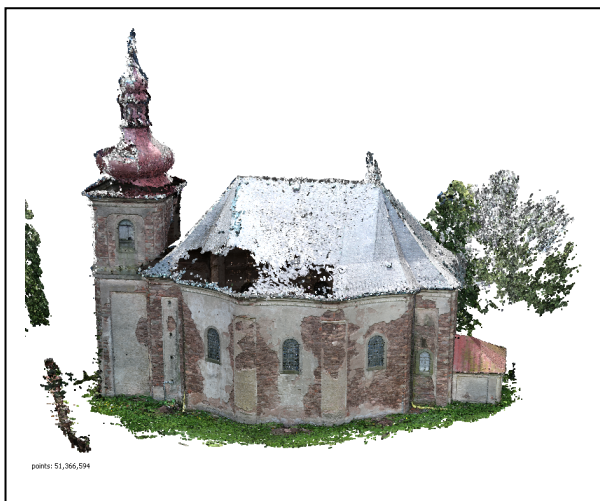
Figure 1. Textured point cloud from terrestrial photogrammetry
