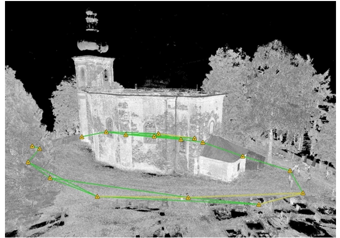
Figure 5. Point cloud from TLS (BLK360, Leica)
