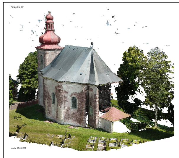
Figure 2. Textured point cloud from UAV photogrammetry
