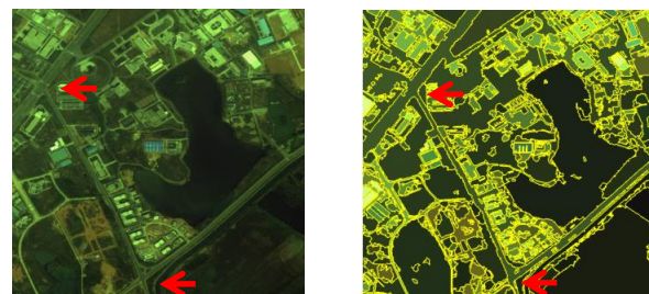
Figure 4. Image segmentation with mean shift algorithm
