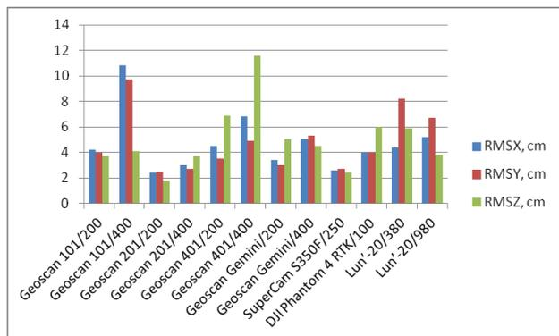
Figure 5. The RMS diagram of the projection centers
