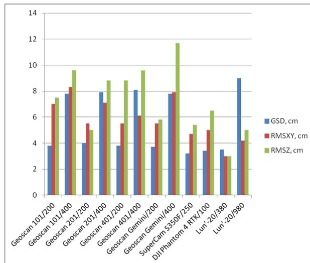
Figure 6. The RMS diagram of the control points after adjustment
