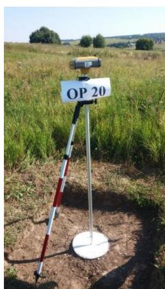
Figure 1. Appearance of the targeted GCP during observation.
