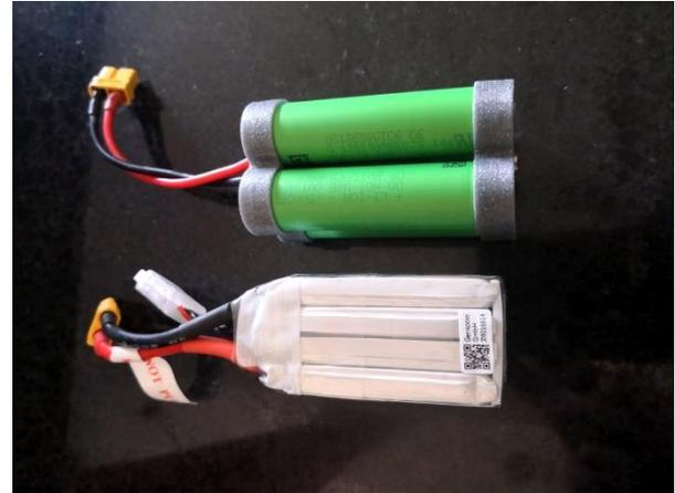
Figure 5: comparison of Lithium Ionic cells and underneath Lithium Polymer pack
