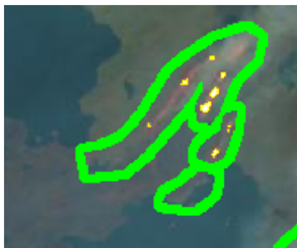
Figure 2. An example of marks. Yellow and white pixels are fire pixels and green pixels are non-fire pixels nearby.
