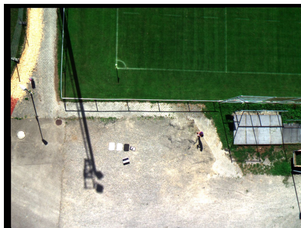
Figure 2. Micasense sample scene with reference panels (true color RGB, 37m sensor altitude).
