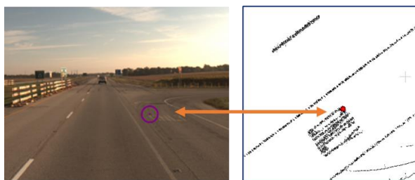
Figure 2. Projection of a location (empty magenta circle) in a RGB imagery onto the corresponding LiDAR Point cloud (red dot) using the estimated LiDAR/camera/GNSS/IMU system calibration parameters
