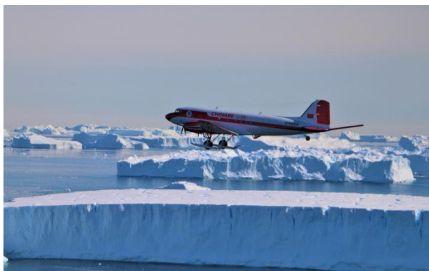
Figure 1. The “Snow Eagle 601” airplane flying over icebergs in coastal areas of Larsemann Hills, East Antarctica. Two flat plate antennas are installed under two wings respectively; the CS-3 magnetometer is installed in the tail boom; the GT-2A gravimeter is installed in the airplane.
