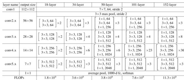
Figure 6. ResNet-50 model architecture (He et al., 2016).
