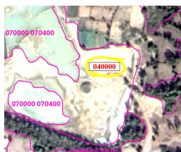
(c) Industrial and mining land (CC2 code is 050200) is misclassified as grassland (CC1 code is 040000).
