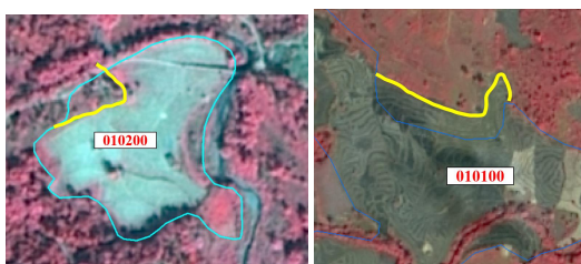
(a)The deviation between the boundary of dry farm patch and the orthoimage is more than 20 meters.
