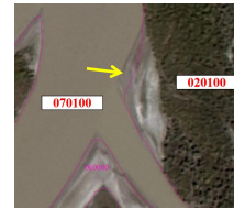
(c)The boundary of the river (CC2 code is 070100) is not edited according to the image.
