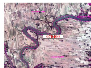
(b) River (CC2 code is 070100) is misclassified as a pond (CC2 code is 070400).
