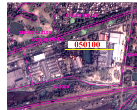
(a) Industrial and mining land (CC2 code is 050200) is misclassified as buildings (CC2 code is 050100).
