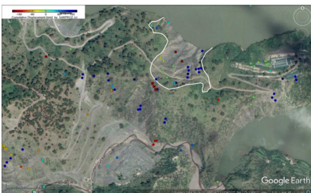
Figure 9. Persistent Scatterers on a Landslide A on the Rim of the Reservoir. Red ones are showing negative LoS displacement whereas Blue ones are showing positive LoS movements
