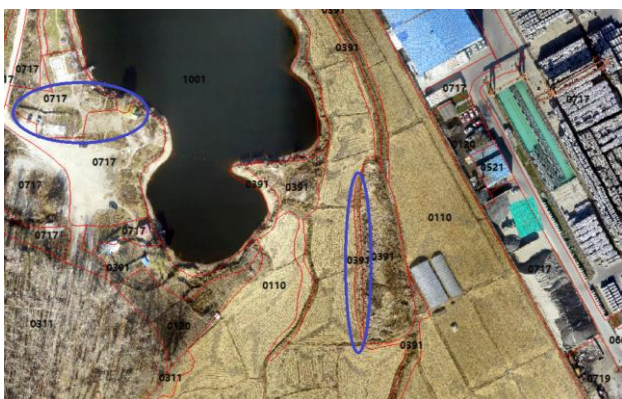
Figure 7. Surface classification data collected by satellite imagery and image overlay obtained by drone
