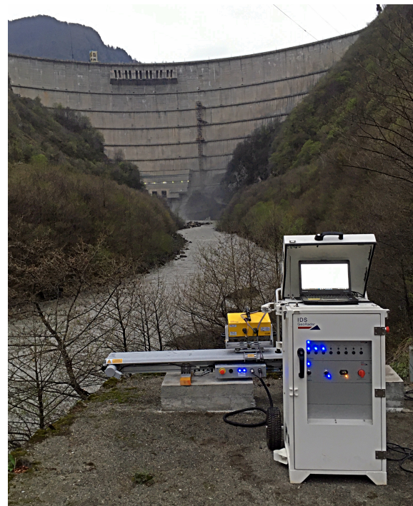
Figure 2. Standpoint of the GB-SAR for the Enguri dam monitoring
