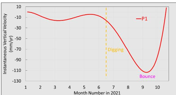
Figure 14. Series of instantaneous vertical velocity of P1 (Figure 12). Mining occurred in middle June.
