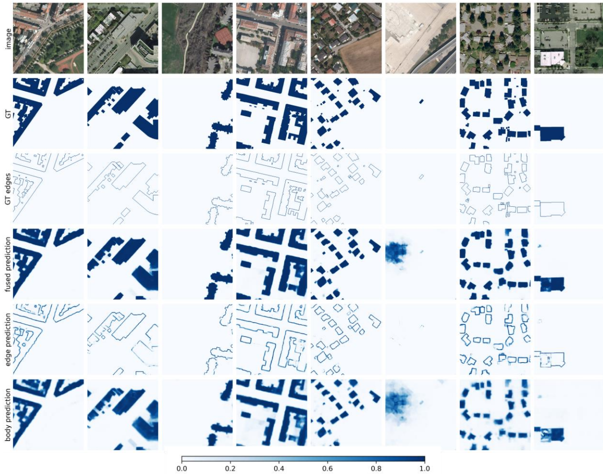
Figure 5. Random image samples together with the ground truth building footprints (row 2) and building boundaries (row 3) as well as the proposed model predictions.
